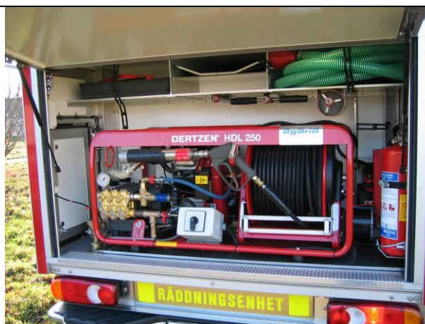
100 m slang, el-slangrulle, 195 l tank
